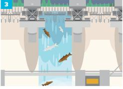
Spillway Entrainment: The passage of fish over a hydro facility spillway happens when there is a need to pass excess water through a dam.
