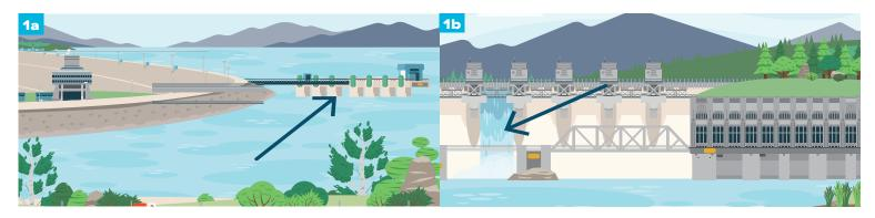
Fish can be entrained when they pass through a dam in several ways including turbines (by way of the intakes) (1a) and spillways (1b).
