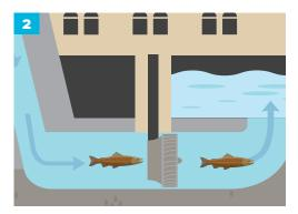
Turbine Entrainment: Fish move through turbines as the generators continuously work to make electricity.
