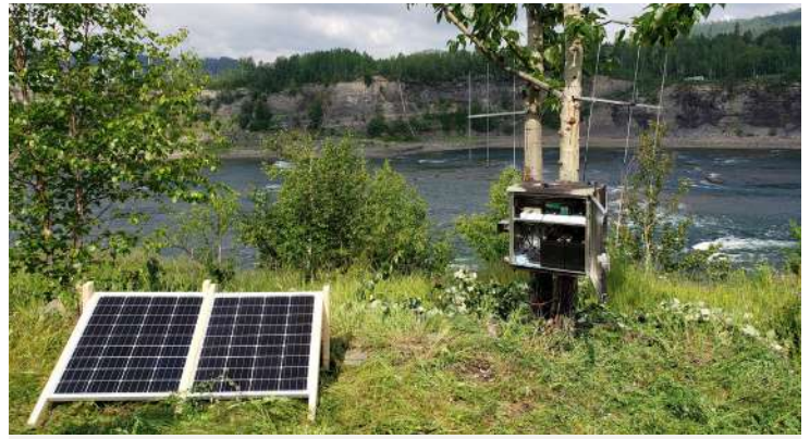
One of 30 new fixed telemetry stations placed on the river bank, which logs data when radio-tagged fish swim by.
